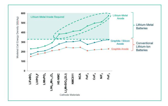
Traditional lithium-ion cells use a hosted anode in which the host material, such as carbon or silicon, provides a structure to hold the lithium. For example, in the case of carbon, it takes six carbon atoms to hold one lithium atom. If, however, an anode of pure metallic lithium were to be used, as shown in the schematic below, all the carbon in the anode could be eliminated and the energy could be stored in a much smaller volume, thereby dramatically increasing the energy density of the cell.
